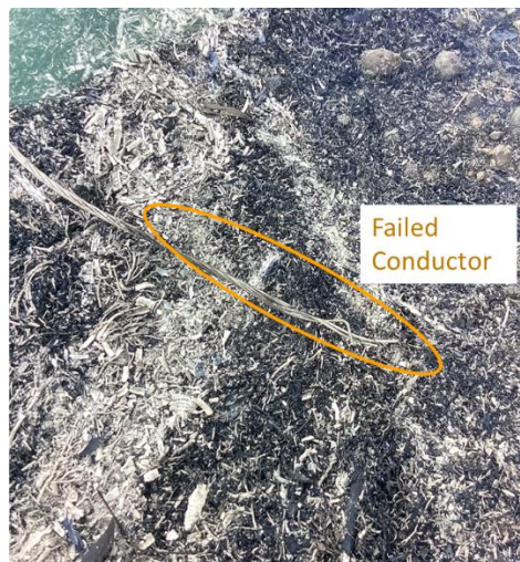
Figure 3. Incident photos taken July 9, 2024 showing failed conductor from Pole SAP ID 101510120 (left), failed conductor on ground (center), and burn area around pole (right).
