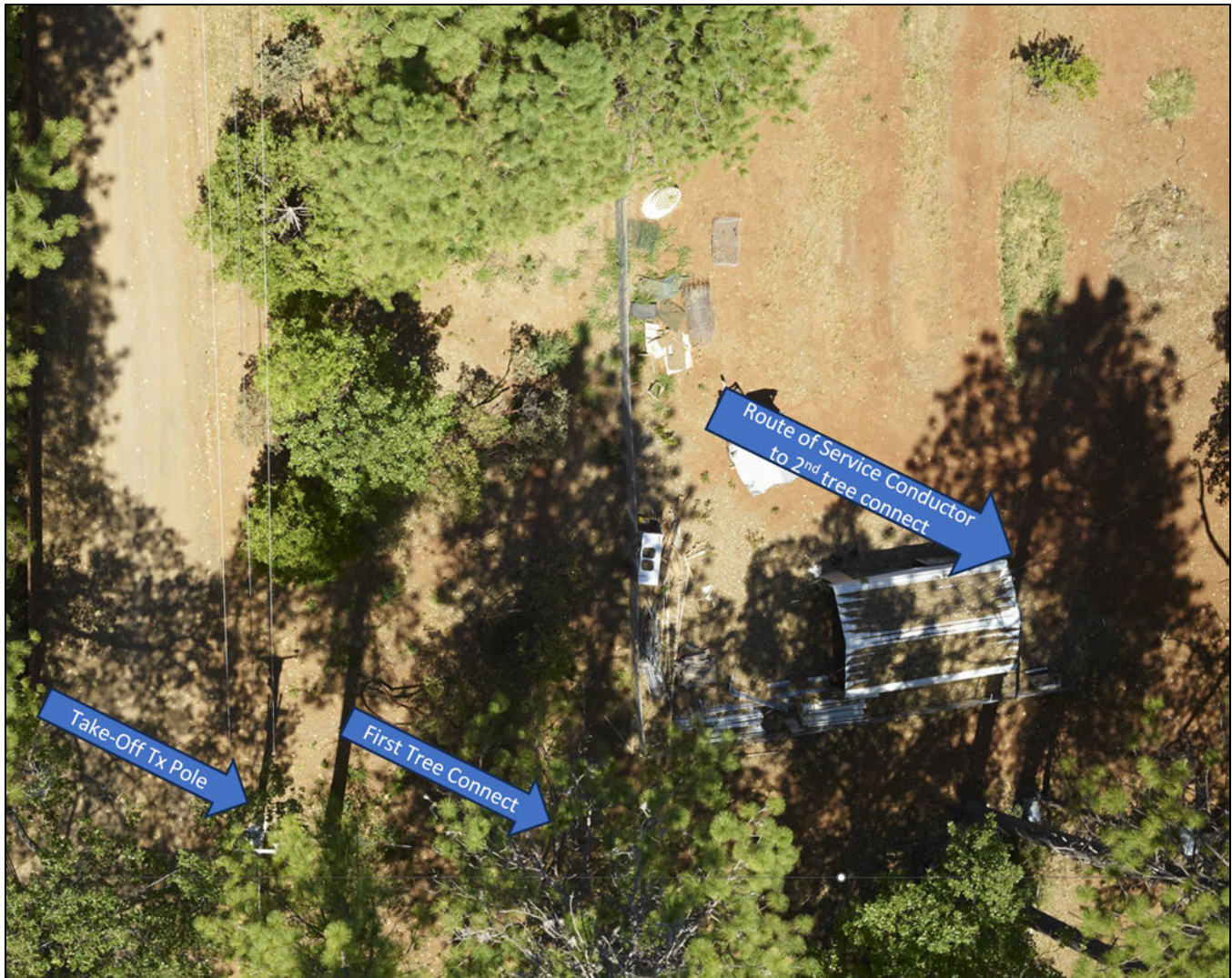
Figure 8 2019 Sharper Shape image showing the route of the service conductor from the Take-Off Tx Pole. 2nd Tree connect is outside of this view to the right.
