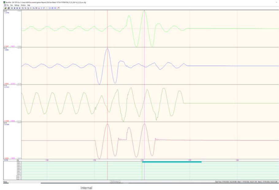
Figure 10 LR 1166 Oscillography showing fault load at time of incident. Source: EPSS investigation report.
