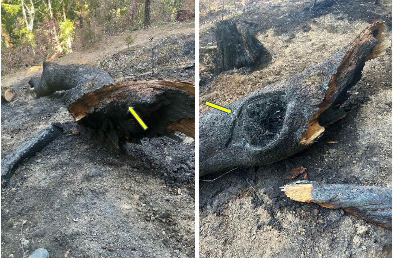
Figure 7 Views of failed trunk. Arrow in the left photograph points to location of apparent internal degradation. Arrow in right photograph indicates location of tree “wound” above failure location. Photograph Source: VM Incident Report (dated July 6, 2024)
