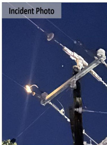
Figure 7 - The vegetation fire was ignited by molten material dripping from a failed H-connector that linked the copper jumper to the Aluminum Conductor Steel-Reinforced (ACSR) conductor.
