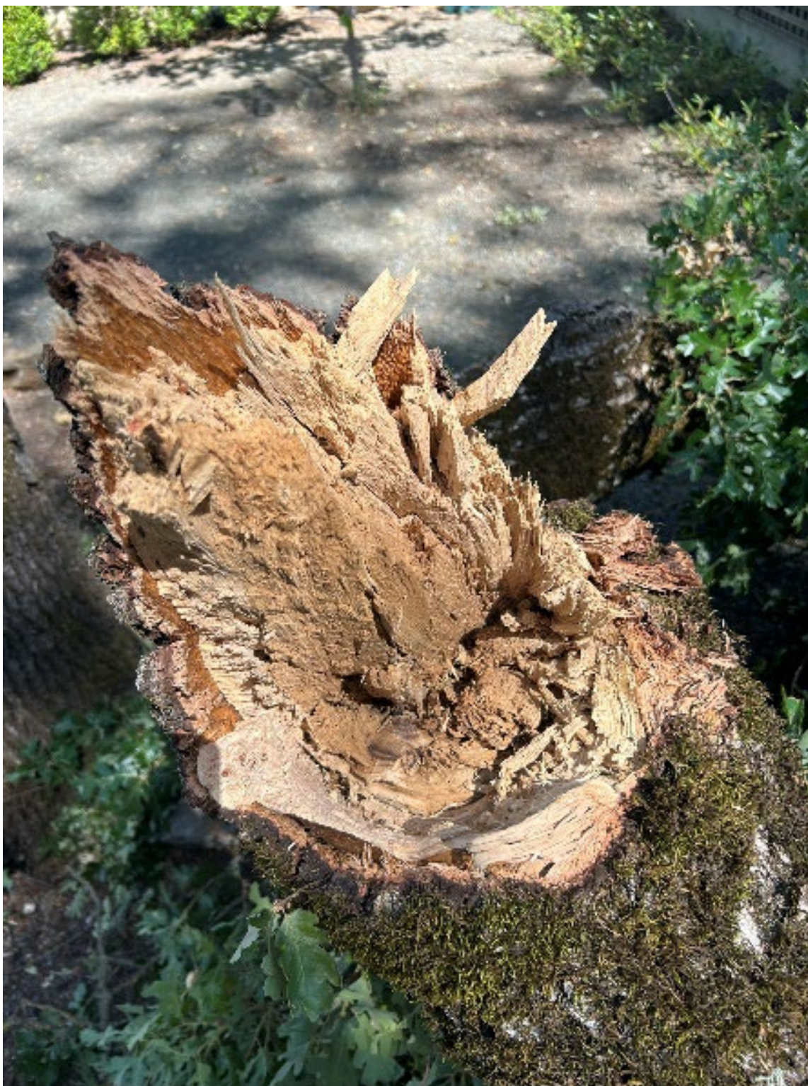
Figure 5: Photo showing the broken end of the branch that caused the ignition. No defect or decay is present in the broken end. Photo collected by VMI.
