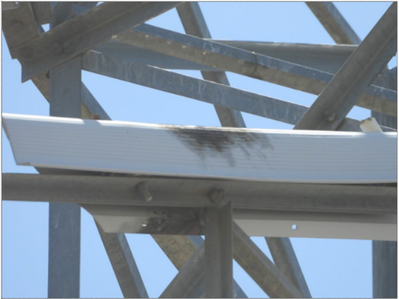
Figure 7 – Photo of burn on bird guard from troubleshooter.
