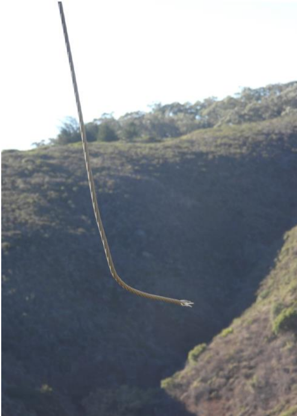
Figure 5 Close up of failed transmission conductor taken by troubleshooter on the date of incident.
