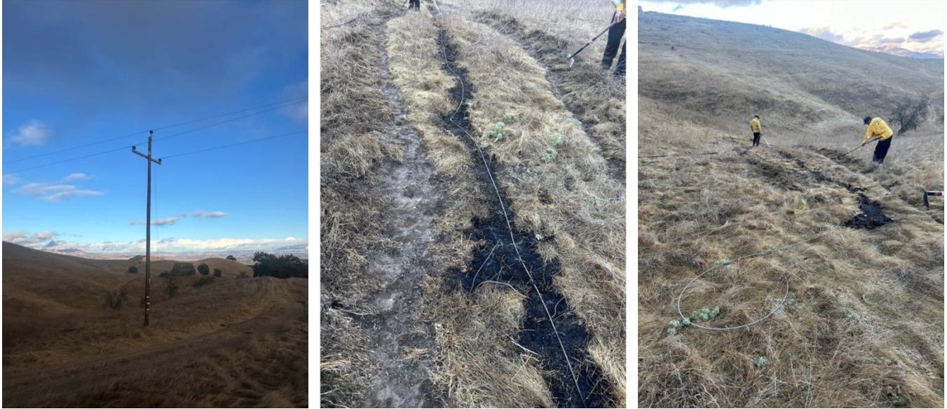
Figure 3. Incident photos showing pole SAP ID 101757232 with broken conductor (left) and burn area (center and right) (taken November 11, 2024).
