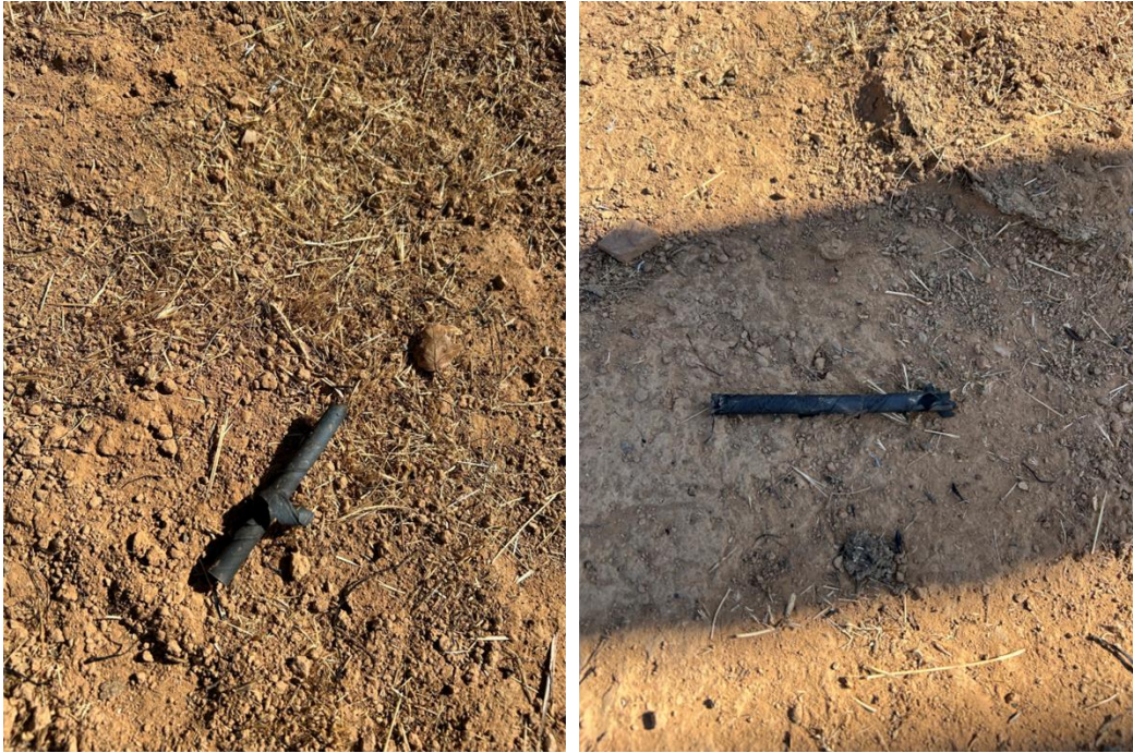
Figure 4. Incident photos showing two burned paper elements of fuse link (taken October 14, 2024).
