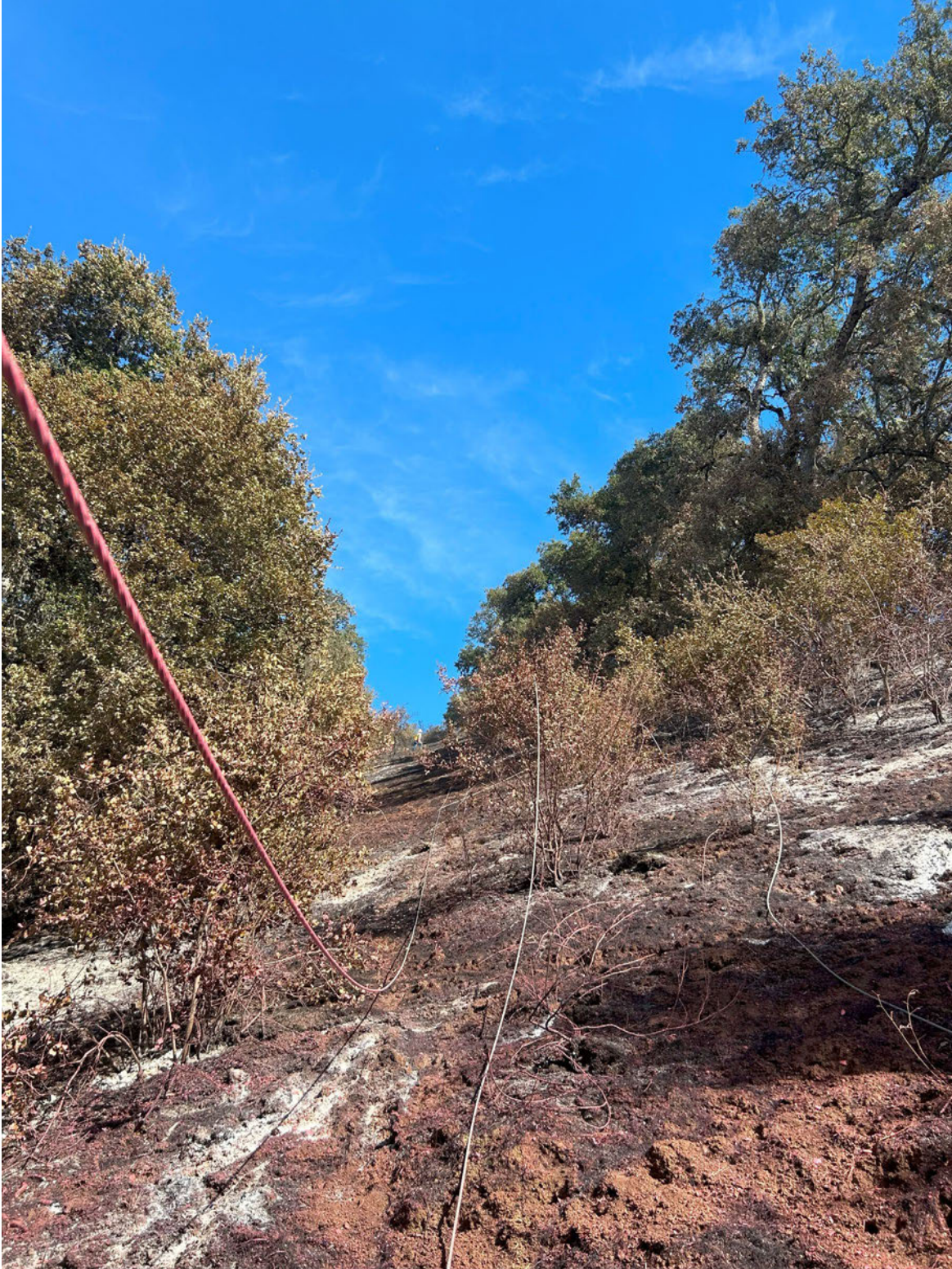
Figure 11: Conductor laying on ground heading looking uphill; photo taken by ignitions investigator October 9, 2024
