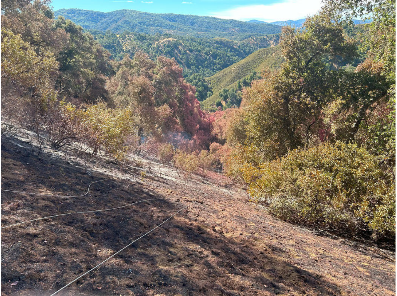
Figure 12: Conductor laying on ground looking downhill; photo taken by ignitions investigator October 9, 2024
