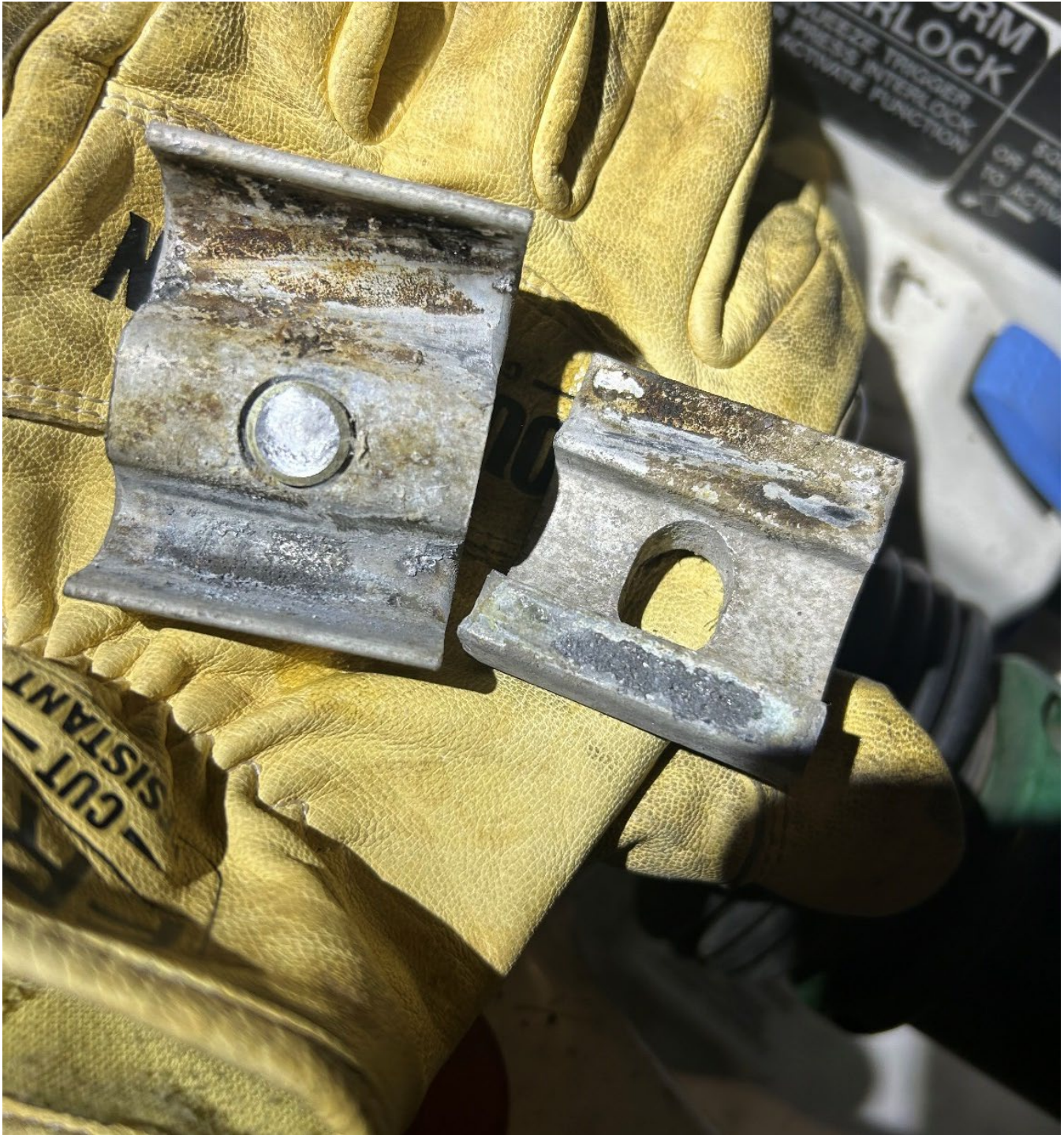
Photo of failed bolt connector at the Incident Location. Photo provided by responding troubleshooter.
