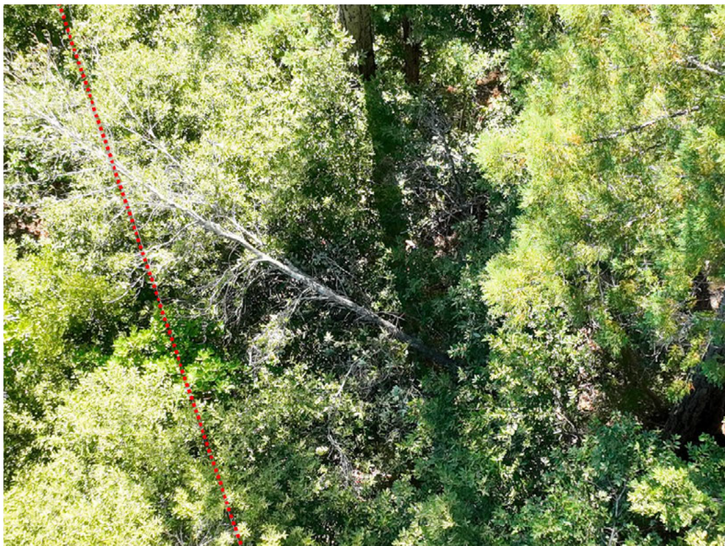
Figure 2 – Incident tree laying across primary line on August 16, 2024 taken via drone. Photo taken by the troubleshooter.
