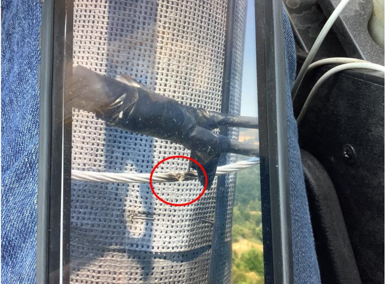
Figure 3 Photo of burn mark on neutral where hot leg made contact taken by troubleshooter on the date of the incident.
