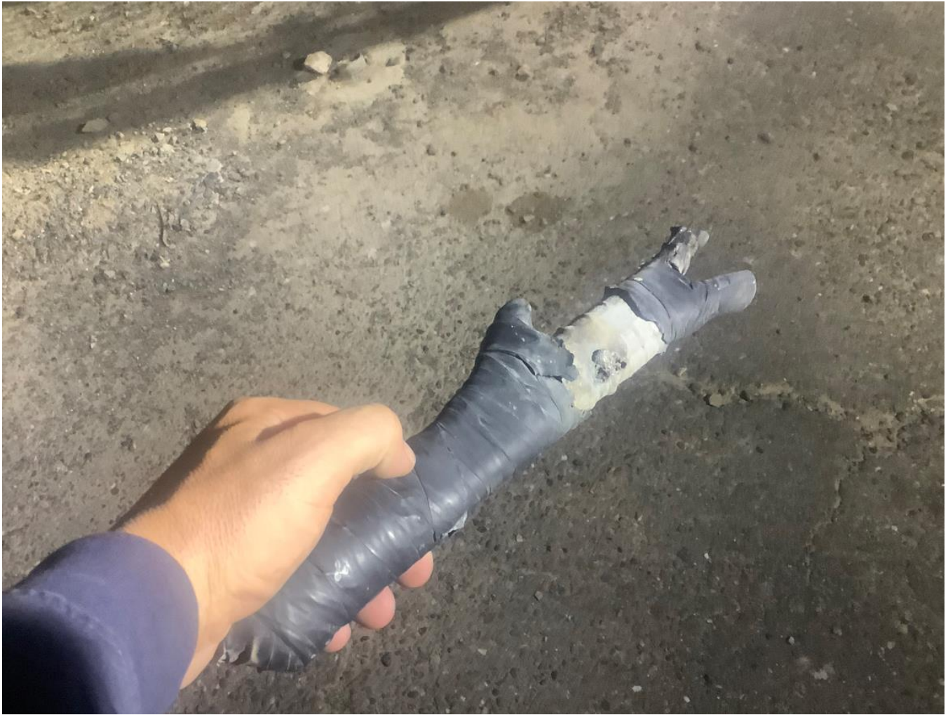
Figure 2 Photo taken by troubleshooter of failed secondary connector.
