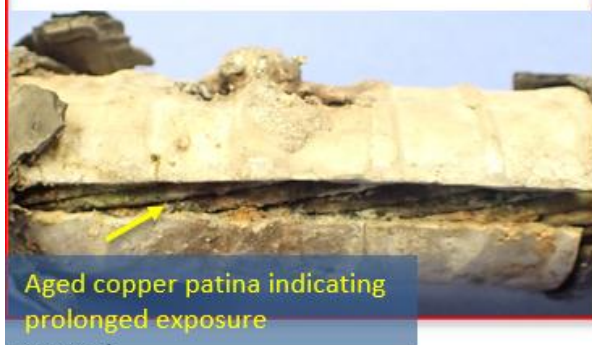
Figure 5 Images taken by ATS of failed connector. CT scan depicted inadequate crimping. Aged copper patina indicating prolonged heat exposure.
