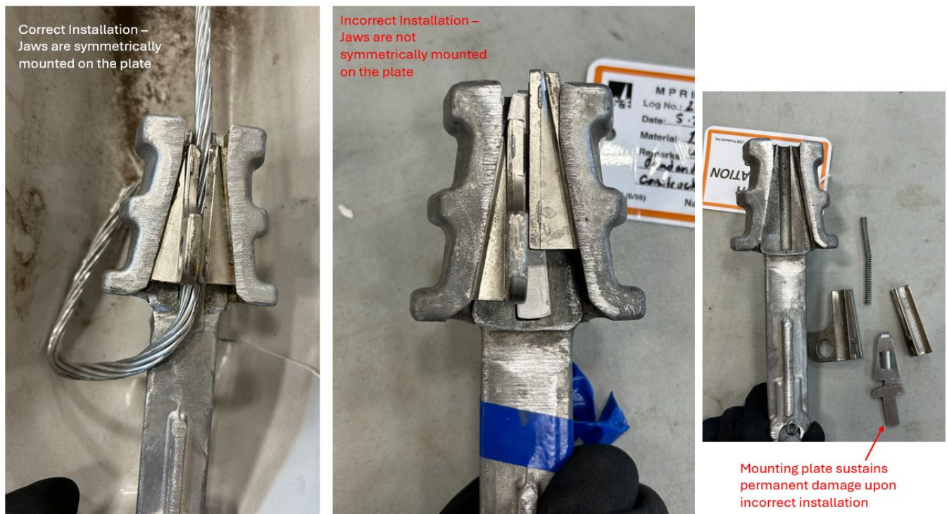
Figure 5 – Replica sample with proper installation (left), incident dead-end shoe assembled by ATS to intentionally show misalignment of components (middle), and mounting plate shown with permanent damage (right). Photos taken at ATS.
