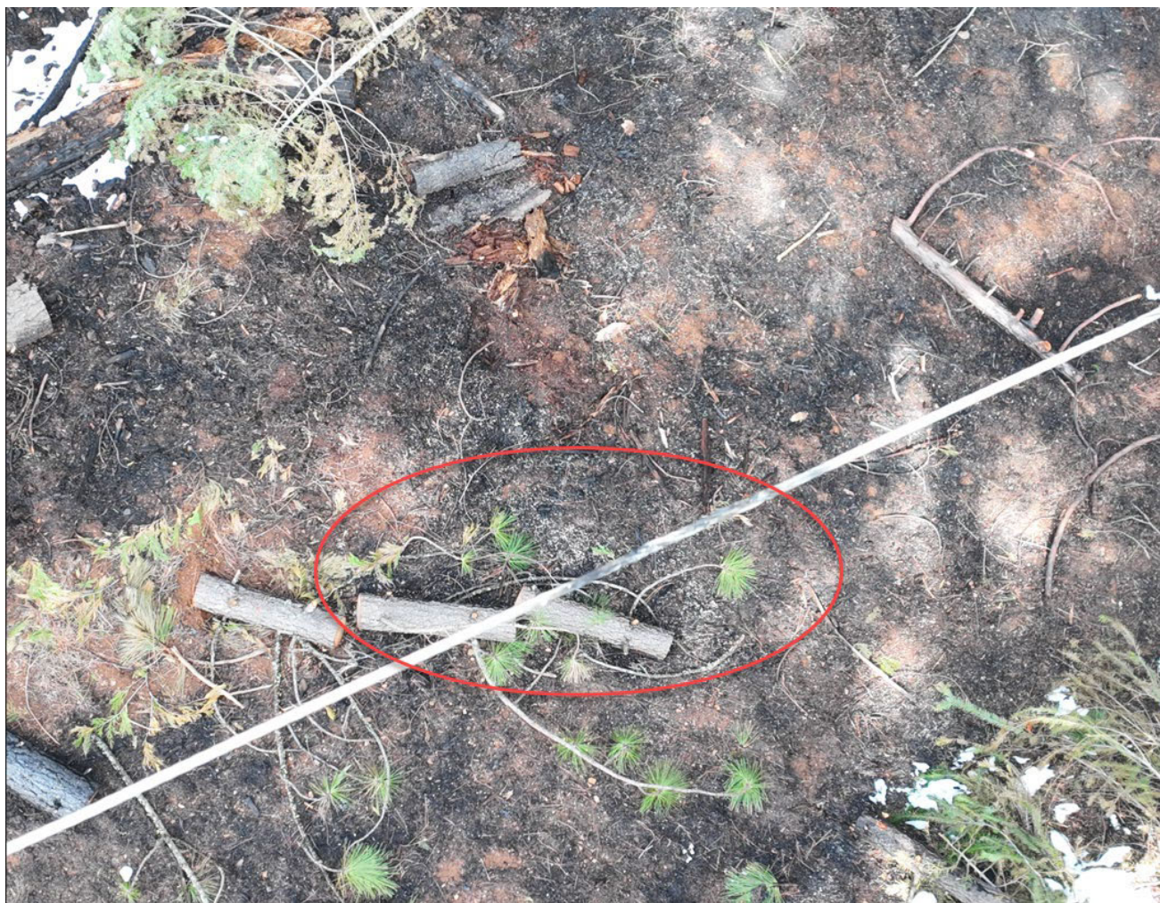
Figure 8 – Image of conductor where tree made contact with the conductor, resulting in the ignition of the fire.
