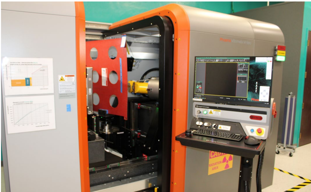
Figure 32. Barrier insulating board positioned inside the X-ray machine.
