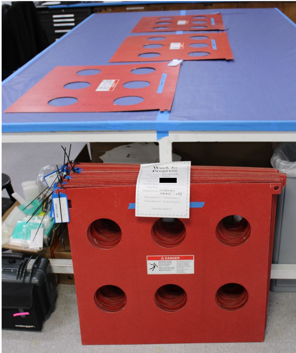
Figure 28. Additional Insulating Boards from the 12 kV bus section of the Mission Substation transferred to Exponent for laboratory examination.
