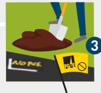
**Use hand tools** at all times when working within 24 inches of the outside edge of any marked underground lines.
