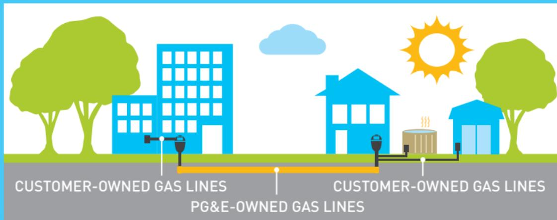
PG&E is responsible for maintaining the system that delivers natural gas, up to and including the gas meter. Customers are responsible for the maintenance of customer-owned piping on their property.
