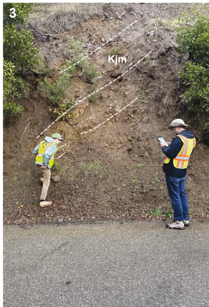
Photo 2: Field Locality 6 – Jurassic diabase/ basalt or graywacke (Jsv/ Jb) with planar, secondary felsic mineralization; Photo 3: Field Locality 7 – dipping beds in the Cretaceous unit (Kjm) directly northeast of linear drainage.
