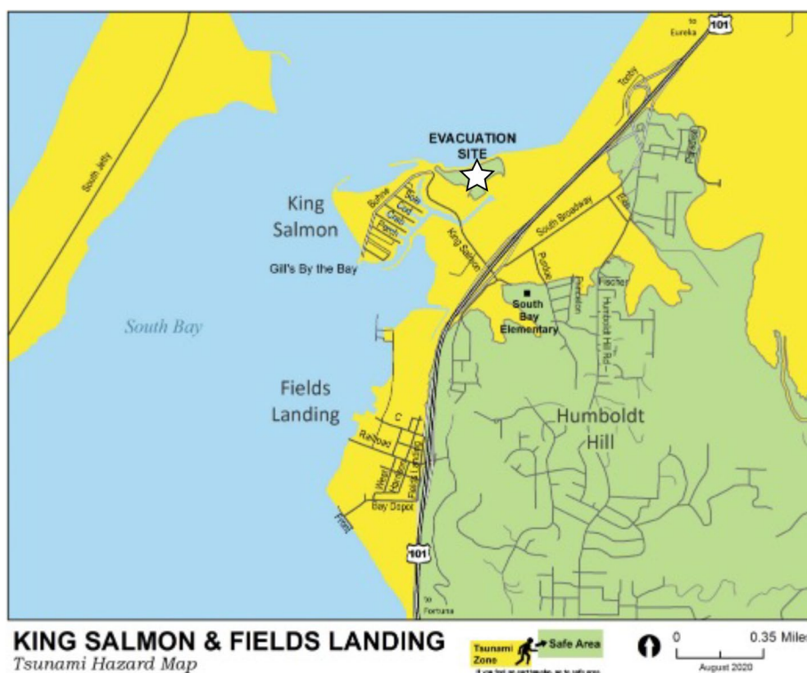
Figure 4 – Tsunami inundation map for King Salmon and Fields Landing (State of California, 2021). This map was produced in association with the Redwood Coast Tsunami Working Group (RCTWG, https://rctwg.humboldt.edu ). Yellow shading indicates areas of inundation. Buhne Hill and the ISFSI site (star) are not inundated in this model and are considered a local evacuation site. Modeling is based Thio (2019).
