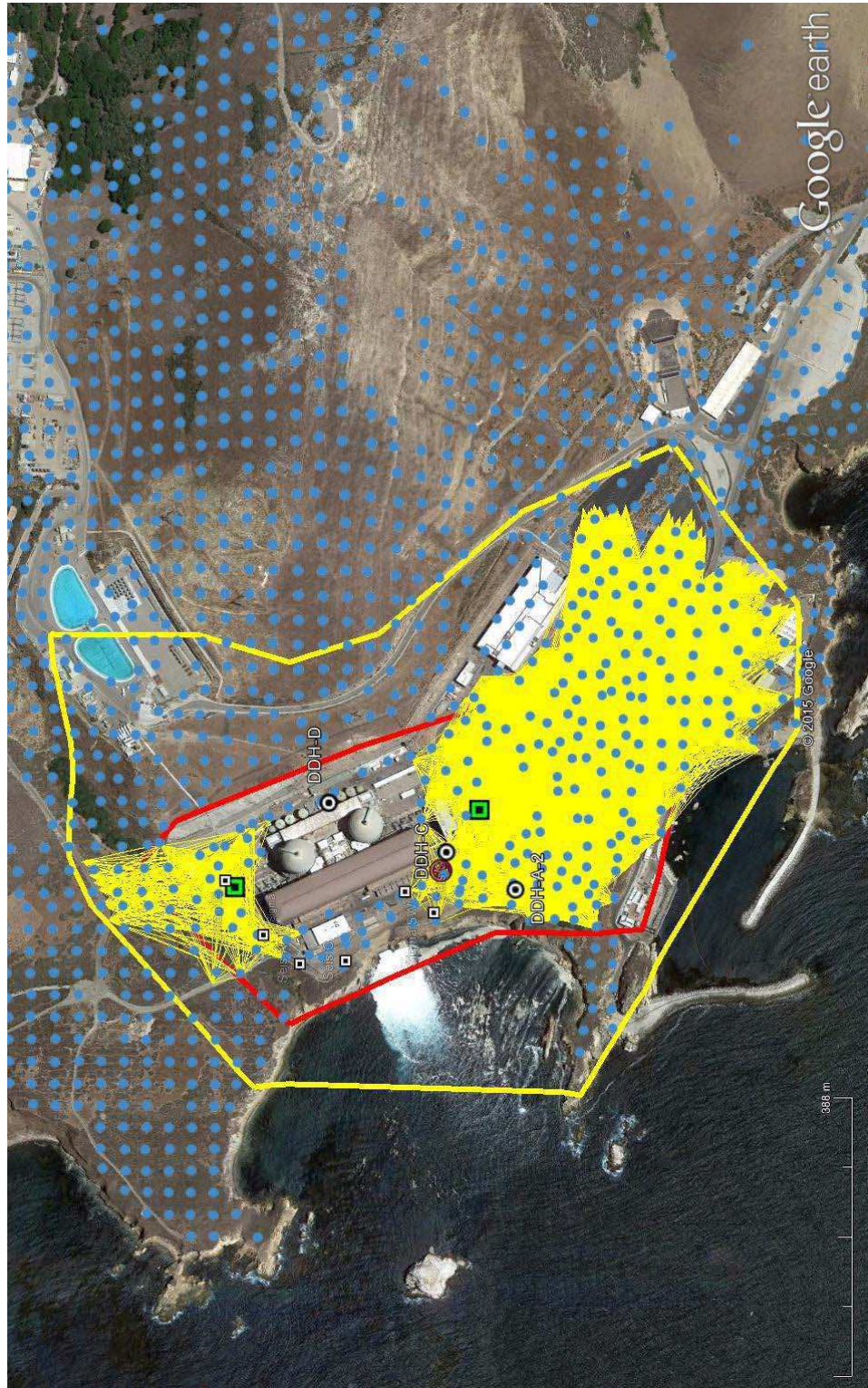
ALL 93 ZLAND RECEIVER GROUP SOURCE-RECEIVER PATHS (YELLOW LINES) (BLUE CIRCLES SHOW LOCATIONS OF INDIVIDUAL ZLAND NODES) Update of the 3-D Velocity Model for the DCPP Foundation Area San Luis Obispo, California
