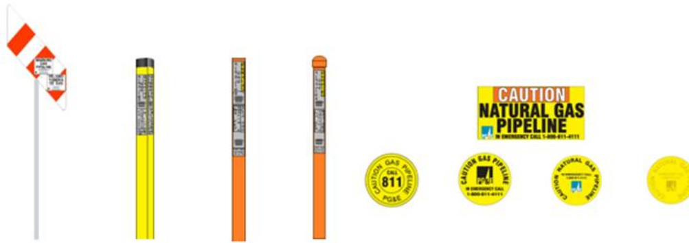
Figure 34 – Types of Pipeline Markers
