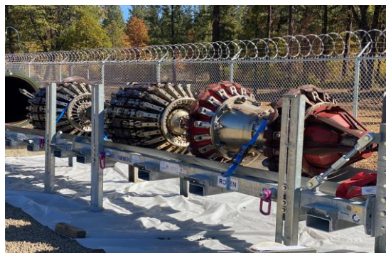
Figure 42 – Electro Magnetic Acoustic Transducer (EMAT) Tool After an Inspection on Line 400
