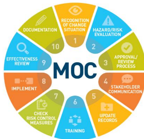
Figure 14 – Gas MOC Process
