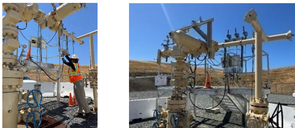
Figure 71 – RD&D Performing Controlled Gas Releases to Test the Viability of the Methane Monitoring System
