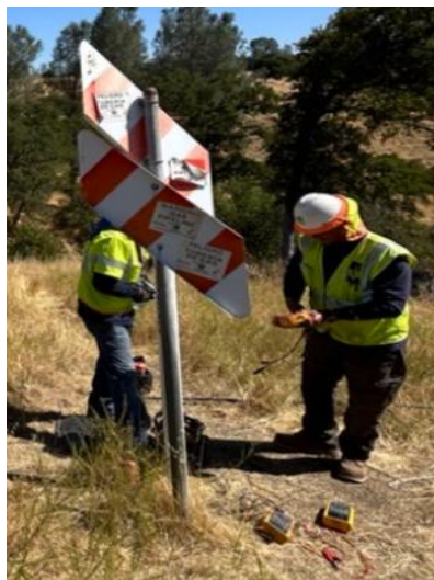
Figure 45 – PG&E Employee Performing Pipe-to-Soil Monitoring
