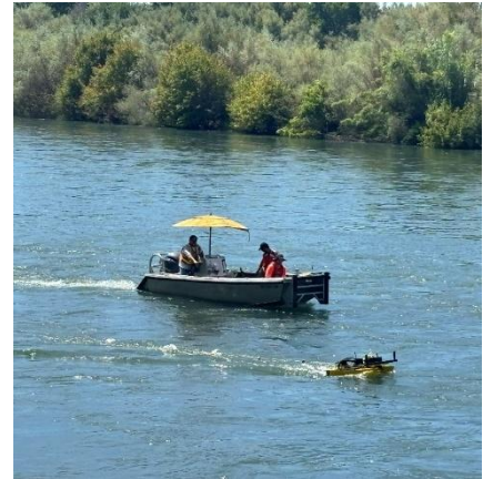
Figure 75 – CMI Non-Intrusive Survey on Boat Platform at Sacramento River Crossing in Red Bluff
