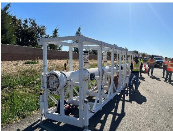
Figure 40 – 12" x 8" pig launcher for the training loop
