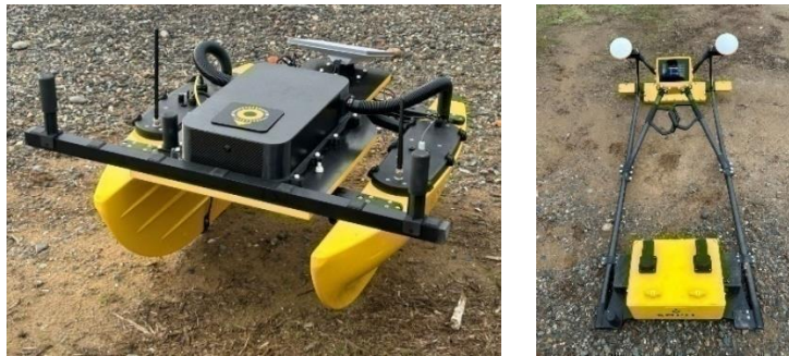
Figure 71 – EMPIT’s CMI with bathymetry sonar on Autonomous Boat (left); Handheld CMI tool (right)
