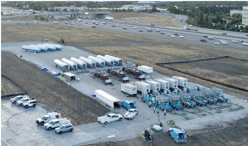
Figure 25 – A Large-scale LNG injection Site in Dublin, CA Supporting a Planned Gas Outage
