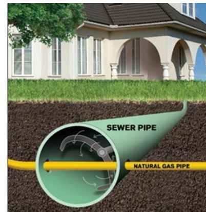
Figure 35 – Cross-Bore
