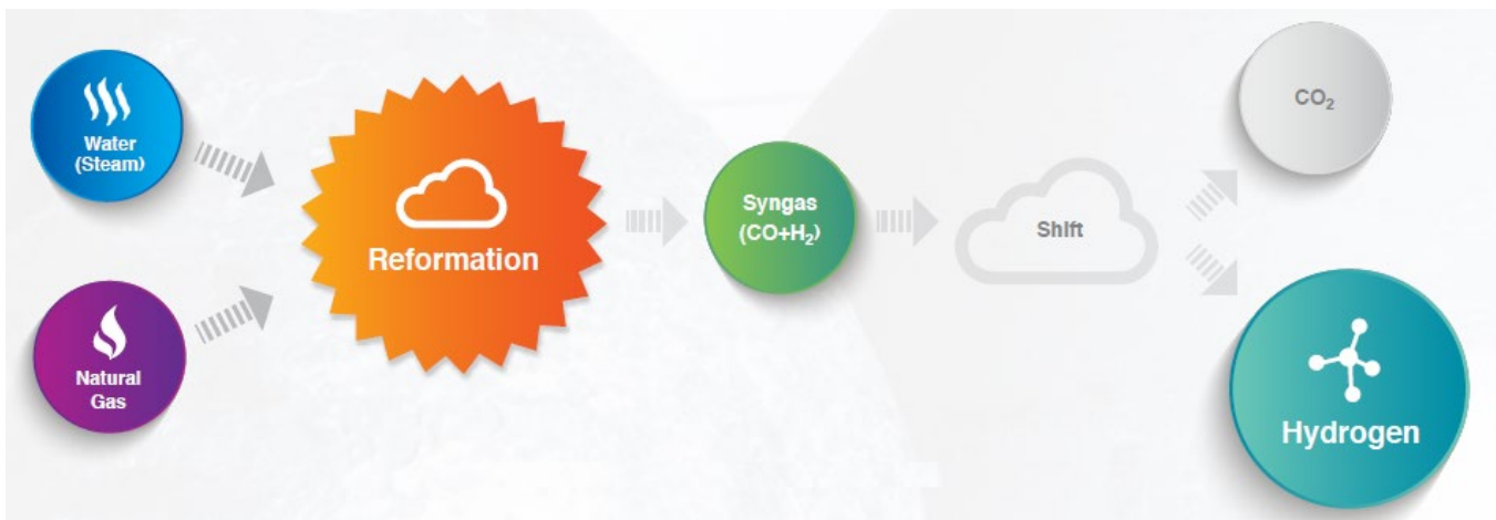
Figure 3 Flow chart of steam methane reforming (South Coast Air Quality Management District (SCAQMD), 2018)
