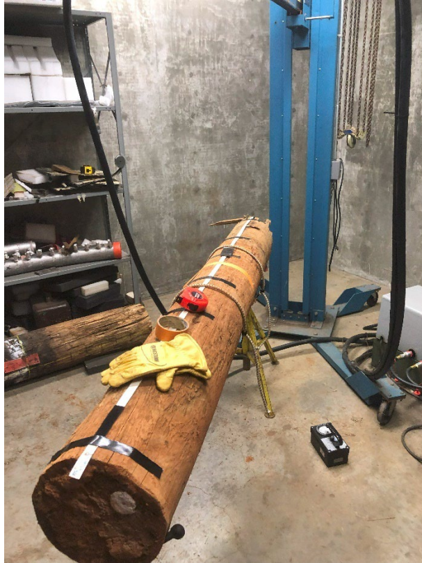
Figure 2 - ATS Radiography Shooting Cell Setup
