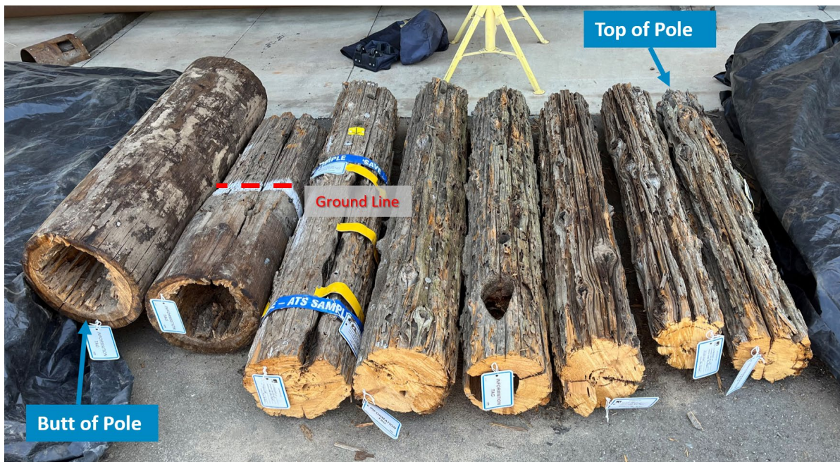
Figure 144 - Pole Sample with Groundline Decay and Woodpecker Hole Damage
