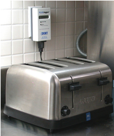
Figure 1: PLUGlogger monitoring energy use of an appliance
