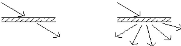
Figure 6. Directional Light Quantified by Luminance and Diffuse Light Quantified by Exitance
