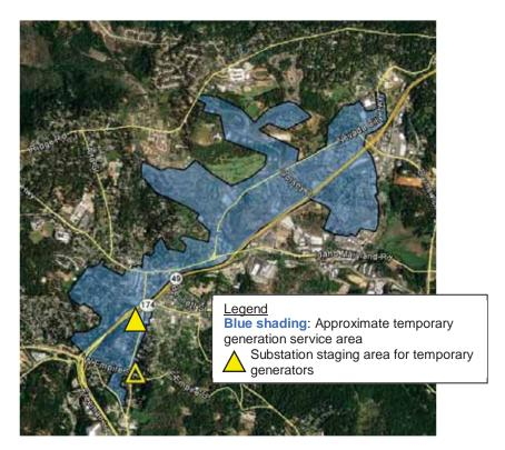
Figure 15: Approximate area served by PG&E Temporary Microgrid in Placerville
