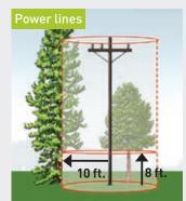
Planting within 10 feet of the base of utility poles and allowing vegetation that can grow more than 8 feet above the ground.
