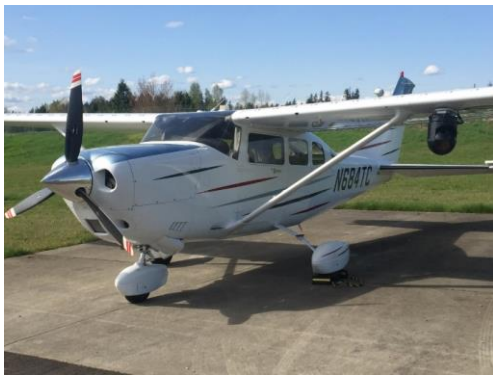
Figure 23 – Patrol Aircraft With Wing Mounted Camera
