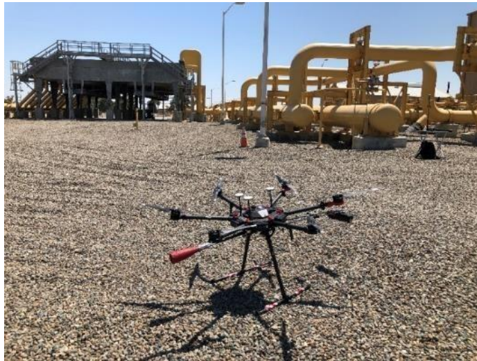
Figure 60 – Drone equipped with RKI’s high sensitivity methane sensor to assess methane emissions at a compressor station
