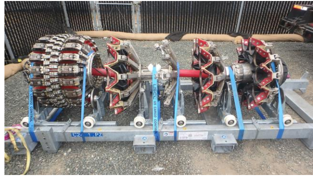
Figure 30 – Electro Magnetic Acoustic Transducer (EMAT) Tool Before an Inspection on L-210C
