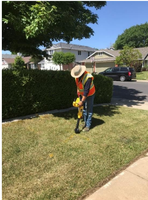
Figure 61 – Using the Vivax-Metrotech GNSS-enabled vLoc3 RTK-Pro locator to collect GPS coordinates of an underground asset
