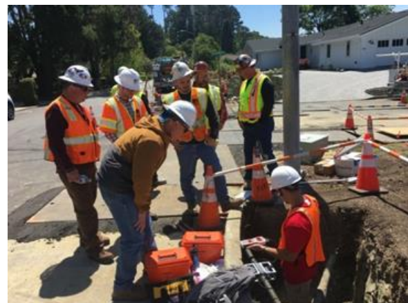
Figure 64 – Field Test of The Plastic Insert Detection Tool
