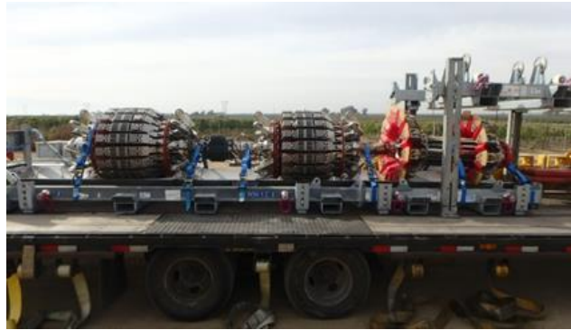
Figure 31 – ROSEN Electro Magnetic Acoustic Transducer (EMAT) Tool Before an Inspection on L-300A
