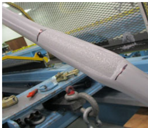
Figure 5 Typical Unacceptable after Sagging Outer Layer Condition
