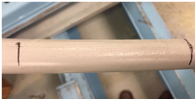
Figure 4 Typical Acceptable after Sagging Outer Layer Condition
