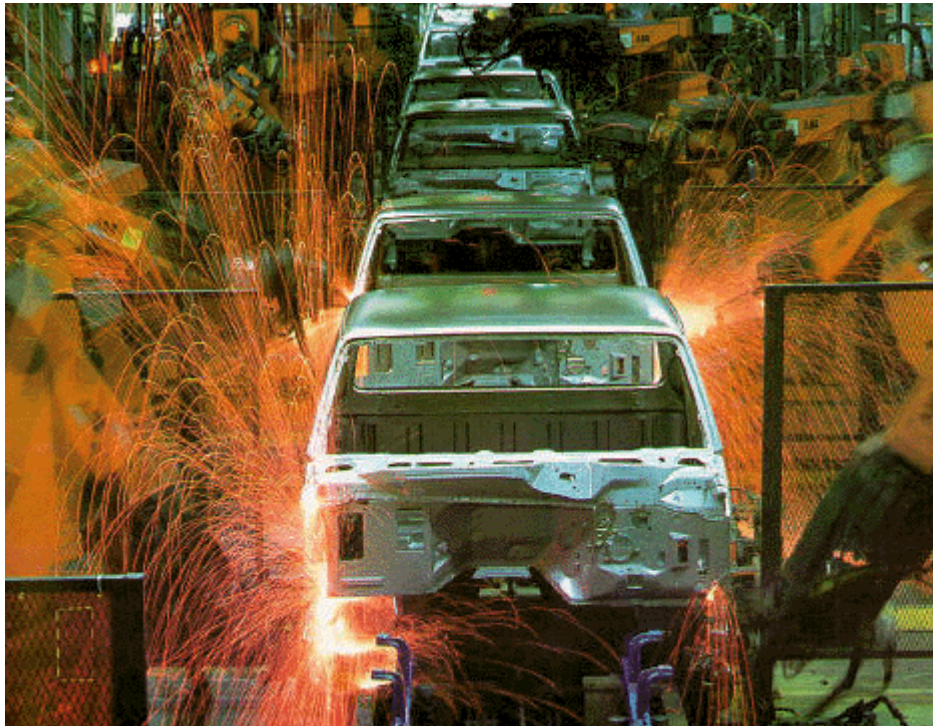
Computer-driven robotics spot-weld truck bodies on Ford's Clayco, Missouri assembly line.
