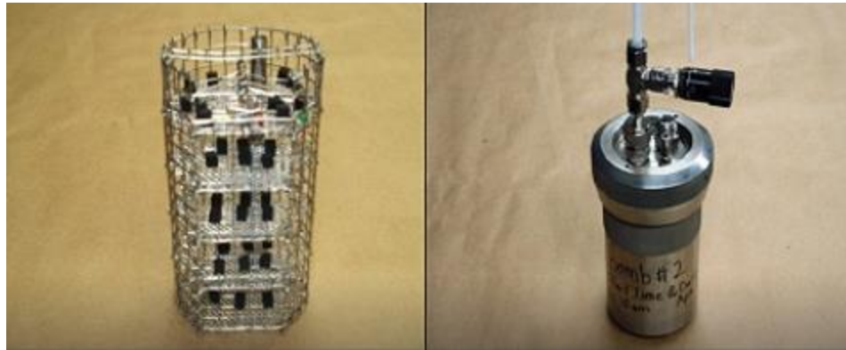
Figure 73 – Elastomer Coupon Test Vessel
