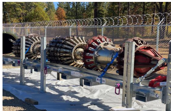
Figure 39 – Electro Magnetic Acoustic Transducer (EMAT) Tool After an Inspection on Line 400
