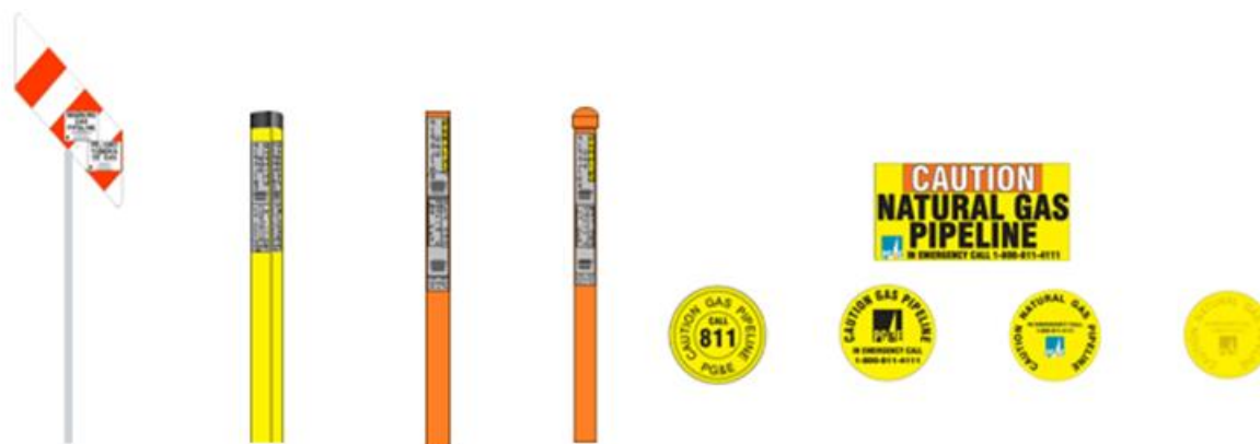
Figure 34 – Types of Pipeline Markers
