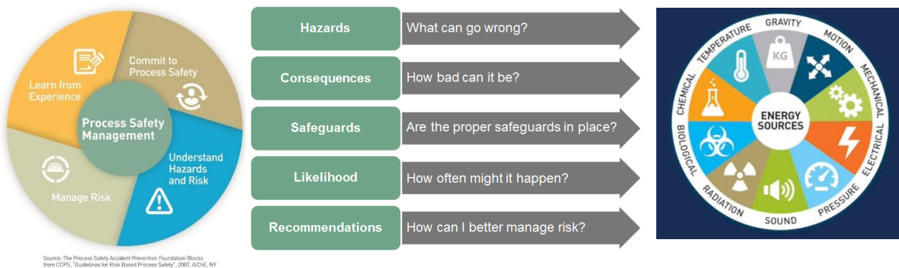
Figure 13 – Gas Process Hazard Analysis (PHA) Process
