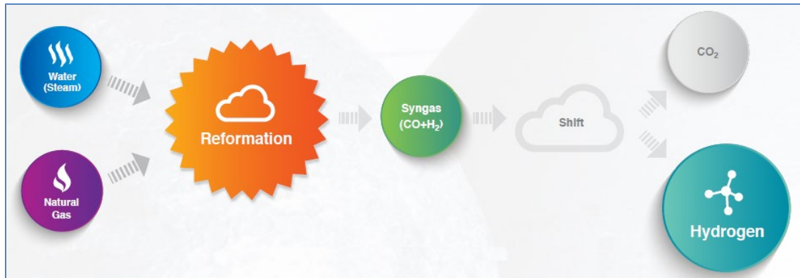
Figure 3 Steam Methane Reformation Path (PG&E R&D and Innovation, 2018)
