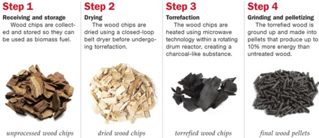
Figure 10 Steps for preparing Biomass (Word of the Day: Torrefaction, 2016)
