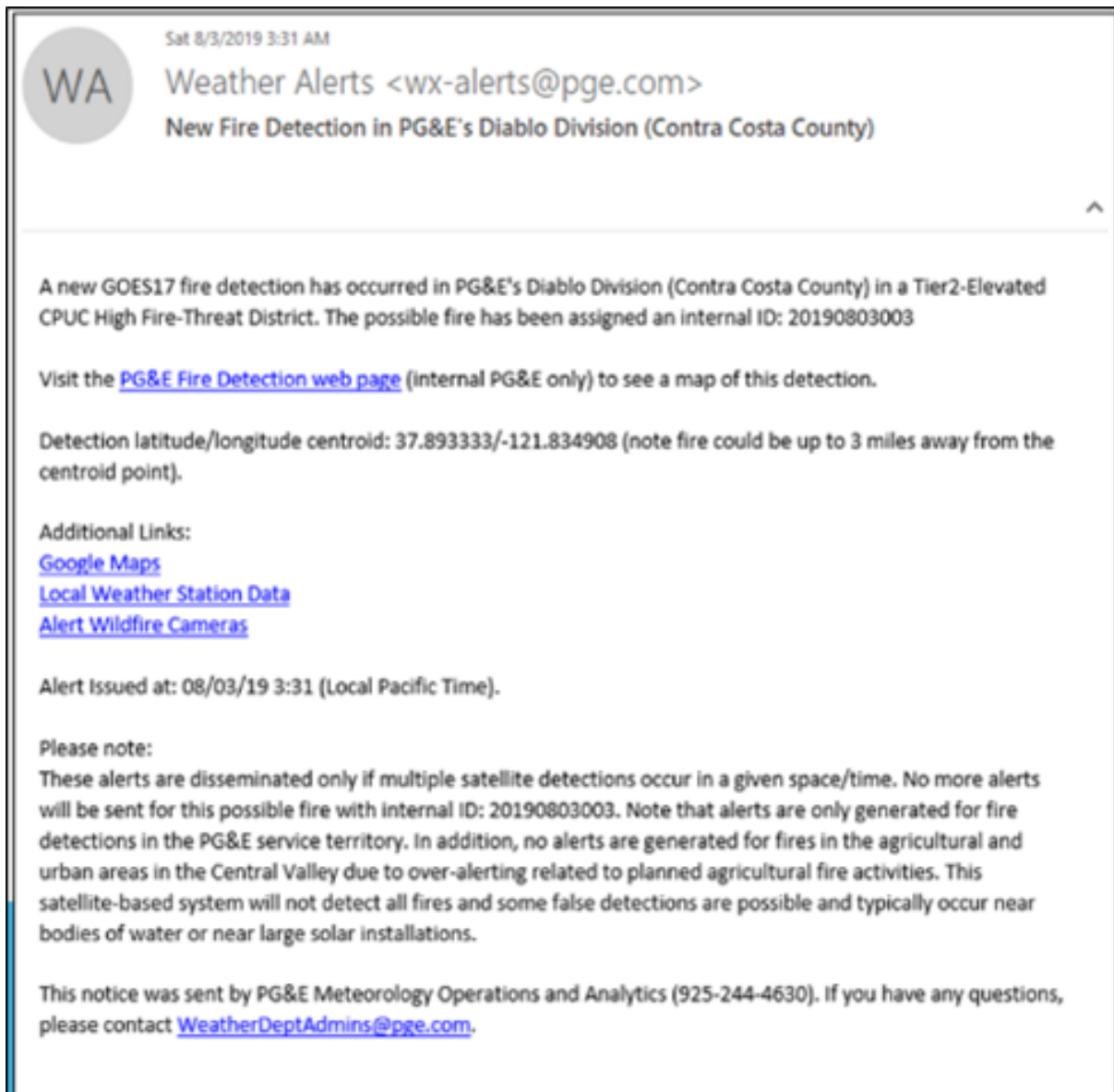
FIGURE PG&E-7.3.2-11: EXAMPLE FIRE DETECTION ALERT EMAIL DISTRIBUTED AUTOMATICALLY BY THE PG&E FDAS – THIS INCIDENT WAS THE MARSH FIRE THAT WAS REPORTED IN CONTRA COSTA COUNTY ON AUGUST 3, 2019
