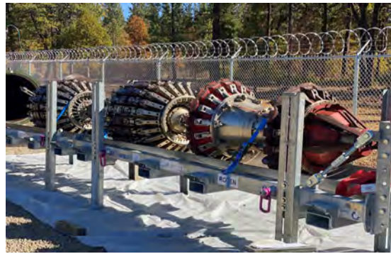
Figure 31 – Electro Magnetic Acoustic Transducer Tool After an Inspection On Line 400
