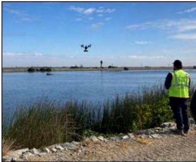
Figure 61 - Water crossing leak survey using an Unmanned Aerial System
