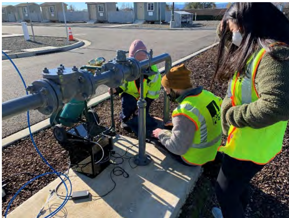
Figure 60 - Test of the novel Mercaptan sensor by UC Davis at PG&E Academy's Winters facility
