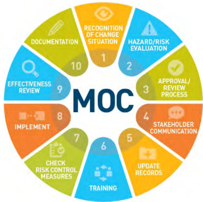
Figure 9 – Gas Operations MOC Process
